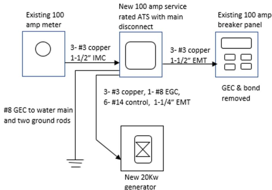
Example of electrical one-line diagram with limited branch circuits:
