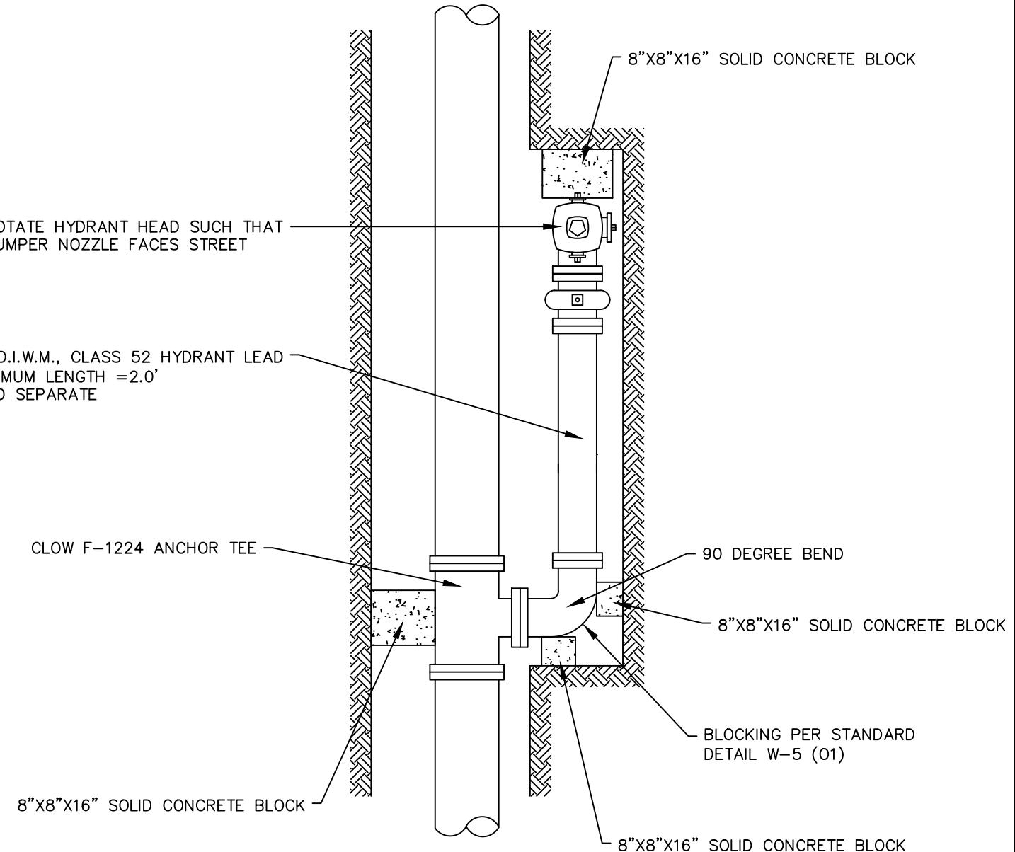
PLAN VIEW FOR INSTALLATION METHOD WHEN PROPOSED HYDRANT LOCATION DOES NOT ALLOW FOR THE INSTALLATION OF A MINIMUM 2' LONG HYDRANT LEAD PERPENDICULAR TO THE WATER MAIN. INSTALLATION METHOD SHALL BE AT THE DISCRETION OF THE ENGINEER.
